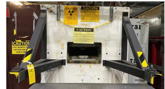
A type 18D72 2.2 Tesla dipole with a 6" gap
