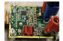
bPOL48V w/ bottom mount heat-sink, 300mH @ 1.5MHz Inductor dimensions: 10 x 12.0 x 7.5mm (LxWxH)
